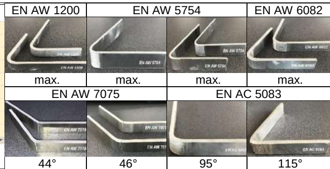
Fig. 6. Specimens of SFSP processed materials, bending tested
