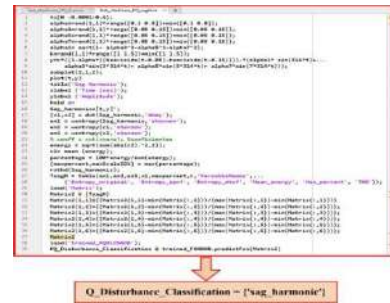
Fig. 10. Result for Fine KNN classifier algorithm with Bayesian optimization using a sag harmonic disturbance signal on input
