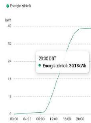
Fig.8. Electricity generated by the bifacial system installed on the rooftop of a residential building.
