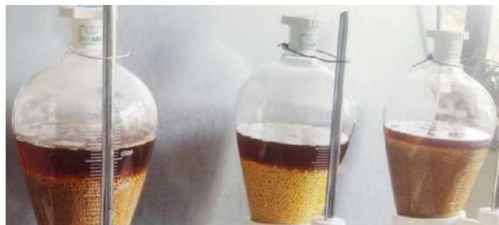
Fig. 3. Initial reactions between oil and adsorbents
