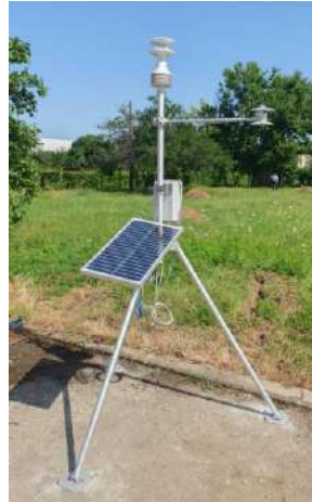
Fig. 2. Weather station equipped with a probe that measures the soil temperature at a given depth
